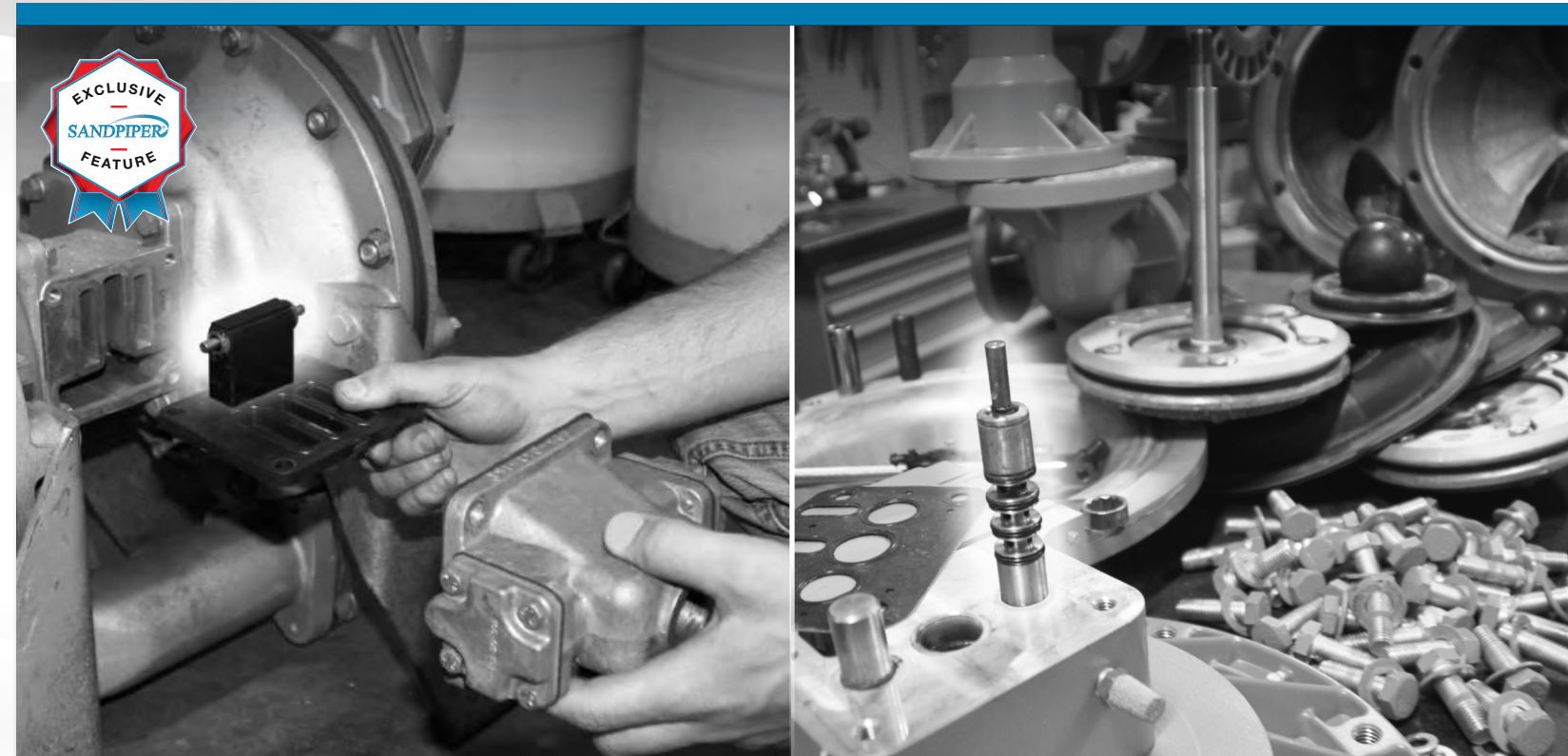
The Air Motor's Pilot Valve is the Most Often Serviced Part on an AODD Pump
