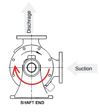
Viking Gear Pump with Clockwise Rotation, Viewed From the Shaft End
