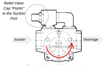
Rotation is the "Long" Way Around from Suction to Discharge
